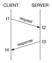
It also calculates and provides, as properties, the round-trip time (rtt) and clock offset estimate (offset) based on this measurement.
