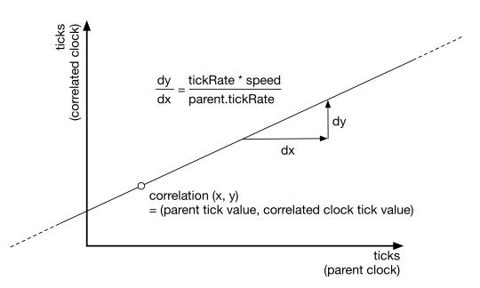
You can alter the correlation and tickRate and speed of this clock dynamically. Changes to tickRate and speed will not shift the point of correlation. This means that a change in tickRate or speed will probably cause the current tick value of the clock to jump. The amount it jumps by will be proportional to the distance the current time is from the point of correlation:
