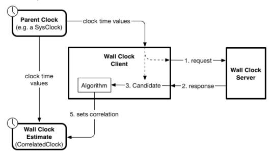
Changed in version 0.4: The measurement process involves taking a reading from the local clock when the request is about to be sent, and when the response is received. This measurement is taken from the *parent* of the clock you provide. The candidate represents a possible relationship between that (parent) clock and the Wall Clock of the server given the results of the request-response measurement. The algorithm processes this and makes a decision as to the *Correlation* that is to be used.
