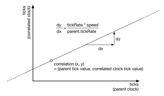
You can alter the correlation and tickRate and speed of this clock dynamically. Changes to tickRate and speed will not shift the point of correlation. This means that a change in tickRate or speed will probably cause the current tick value of the clock to jump. The amount it jumps by will be proportional to the distance the current time is from the point of correlation:
