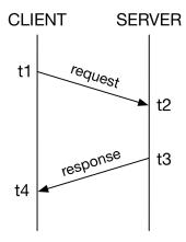
It also calculates and provides, as properties, the round-trip time (rtt) and clock offset estimate (offset) based on this measurement.
